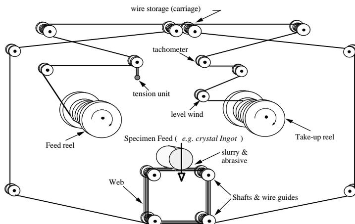
Figure 1. Conceptual wire saw slicing setup
